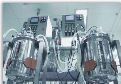
CulNet system (Circulating bioreactor system)
