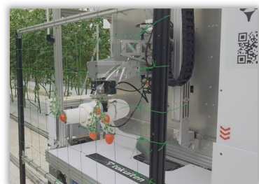
Automated suction-type harvesting robot for mini tomatoes
